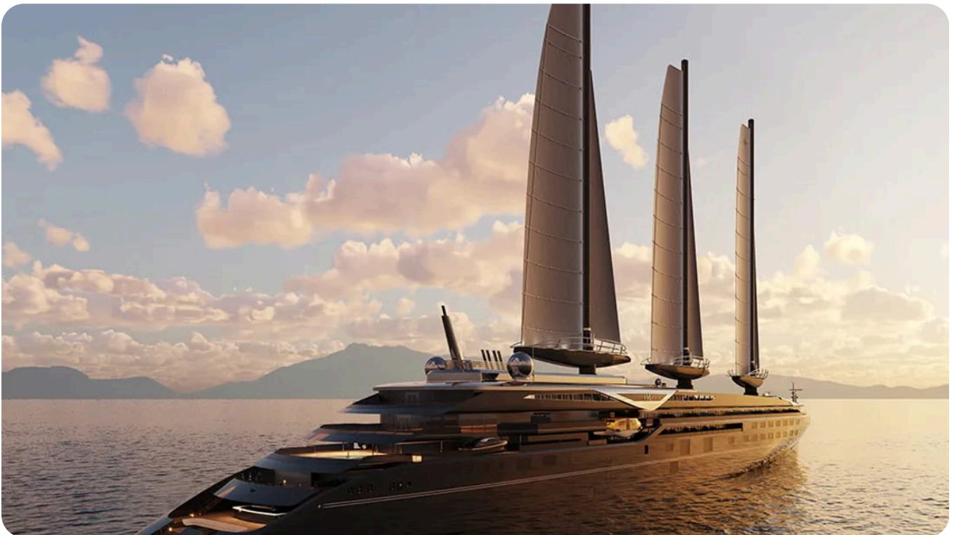
Orient Express Corinthian under sail. Three rigid sails over 100 metres high can provide up to 100% of propulsion in favourable conditions.
